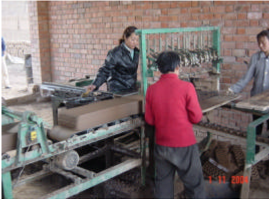
Picture 5: Brick making operations on new production line, Brick plant near Xi'an; (Ref.: TVE project Phase II, PSN 2).
